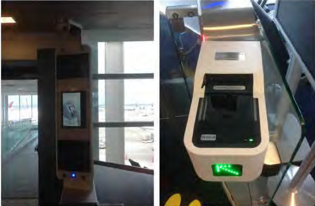
Figure 8. Left: Display screen to illustrate boarding procedure; Right: Boarding scanner
