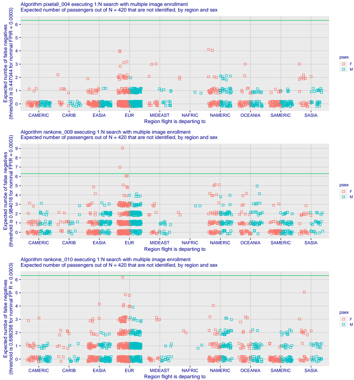
Figure 18: For the eleven regions and two sexes, each point give the expected number of false negatives for a simulated flight in which 420 passengers, 210 men and 210 women, attempt boarding after being enrolled with multiple images each. The numbers are stated by scaling measured numbers of false negatives to 210 per sex. The points' positions are jittered horizontally and vertically to mitigate over-plotting invisibility. There are many more flights to Europe, particularly, and East Asia simply because of their representation in the EXIT image corpus we have. The number of individuals in the gallery is exactly 420.
