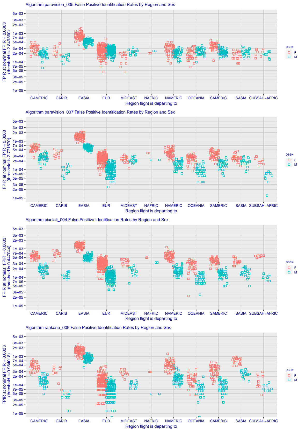
Figure 26: For the eleven regions and two sexes, each point give the false positive identification rarte for a simulated flight in which 420 passengers, 210 men and 210 women, attempt boarding after being enrolled with multiple images each. The points' positions are jittered horizontally to mitigate over-plotting invisibility. There are many more flights to Europe, particularly, and East Asia simply because of their representation in the EXIT image corpus we have The number of individuals in the gallery is exactly 420.
