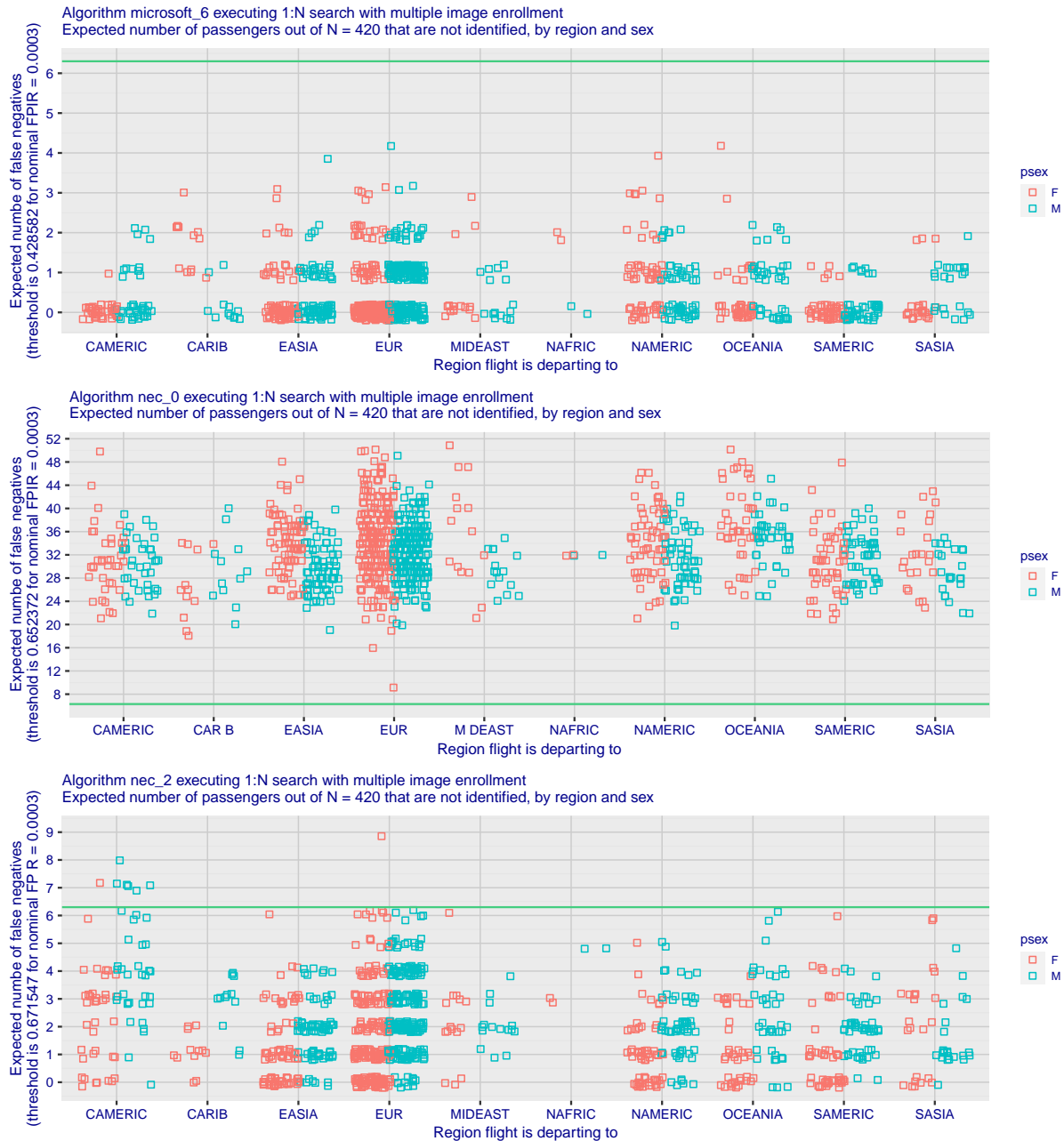
Figure 15: For the eleven regions and two sexes, each point give the expected number of false negatives for a simulated flight in which 420 passengers, 210 men and 210 women, attempt boarding after being enrolled with multiple images each. The numbers are stated by scaling measured numbers of false negatives to 210 per sex. The points' positions are jittered horizontally and vertically to mitigate over-plotting invisibility. There are many more flights to Europe, particularly, and East Asia simply because of their representation in the EXIT image corpus we have. The number of individuals in the gallery is exactly 420.
