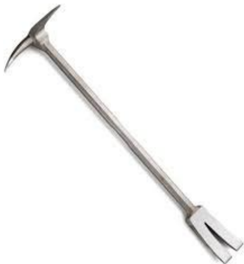
Figure 2-4. Example of a Halligan bar
