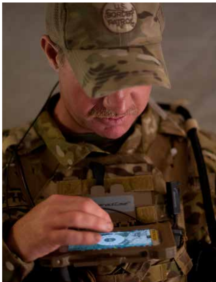
BORTAC agent assesses the Android Tactical Assault Kit during an exercise at Camp Blanding, Florida. Using smartphone technology, the device is reinforced to function in rugged field conditions and shows law enforcers a geographical depiction of their surroundings using interactive moving maps, video, voice and text. Photo by Jeffrey Swenson
