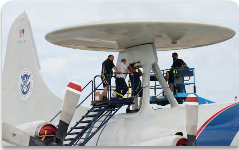
PHOTO: Maintenance contractors re-attach the roto-dome radar package on a P-3 aircraft undergoing SLEP upgrades in Fiscal Year 2016.
