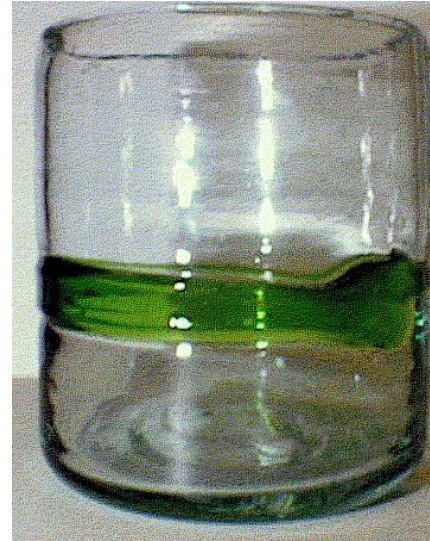
Fig. 6 -Glass Ribbon Effect? Yes. Glass ribbon inserted prior to solidification to create the band or ribbon
