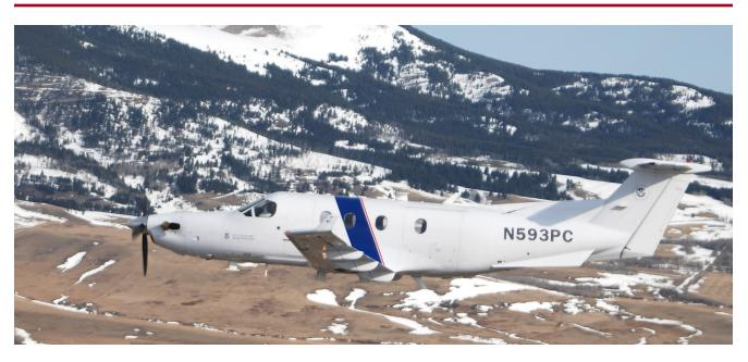
The Pilatus PC-12 is a single-engine, turbo-prop, fixed-wing aircraft used by U.S. Customs and Border Protection, Air and Marine Operations (AMO) that combines the slow-speed capability of a Cessna 210 with the payload and high-speed of a B-200 King Air.
