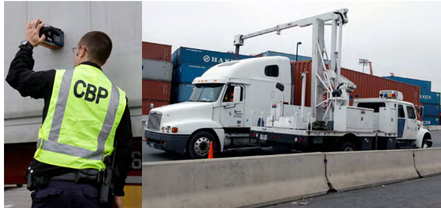
CBP NII technologies include Vehicle & Cargo Inspection System, a truck-mounted gamma-ray imaging system, and Buster, handheld device used to scan vehicles for hidden contraband.
